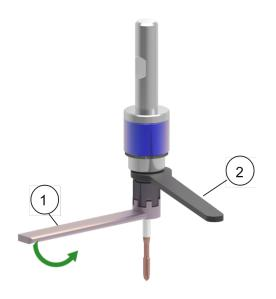
4. Tighten the clamping nut with the appropriate wrench.
