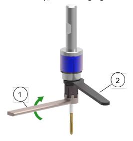
1. Remove the clamping nut with wrench
